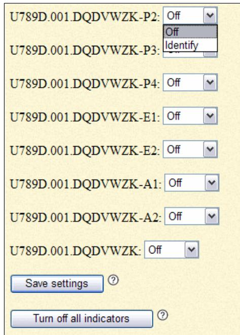
Figure 14-32 Enclosure Identify window
